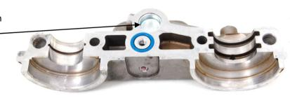
To stop the oil feed, an M6 tap is used to cut a thread in the hole seen above. After thorough cleaning, the supplied grubscrew is then installed with the use of a thread locking compound.
