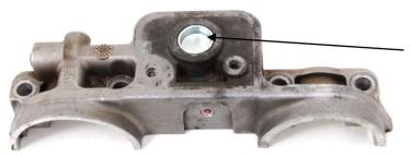
Once the VVT solenoid has been removed, the sealing plugs need to be installed to blank off the hole. One is pressed in flush on the top of the cam bridge.
